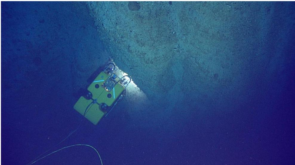
**Fig. 5:** Remotely operated vehicle Hercules examines a vertical pumice wall in the crater of Kolumbo submarine volcano.
