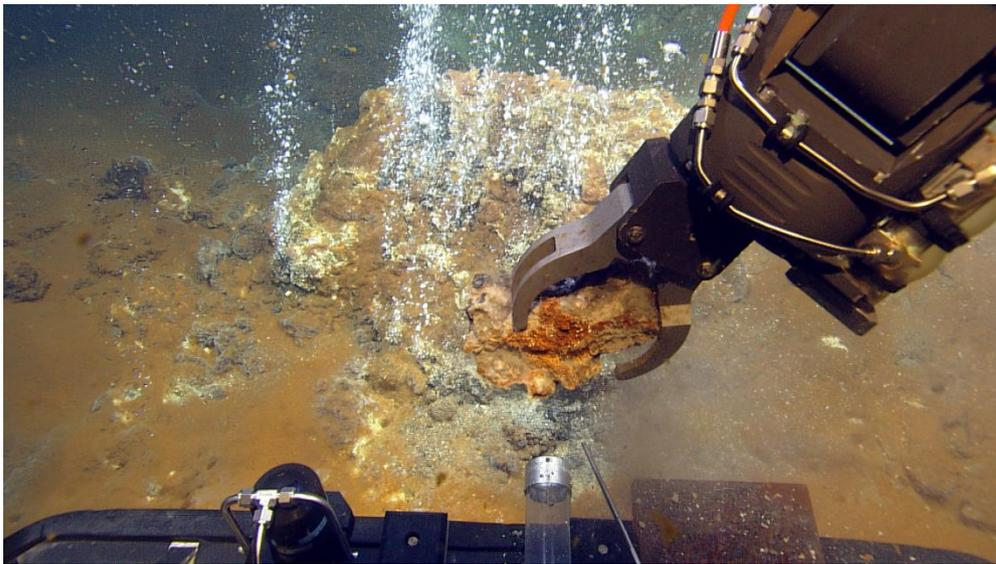
**Fig. 2:** Sampling with the manipulator arm of ROV Hercules from a hydrothermal vent mound discharging both fluids and gases (220°C).
